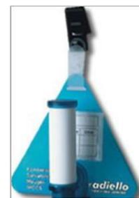
Figure 1 : tube passif (type Radiello)
